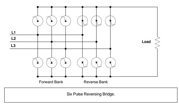
The figure above illustrates a six pulse reversing SCR phase angle controller. When the gates on the forward bank are activated, the current flow through the load is clockwise. When the gates on the reverse bank are activated, the current flow through the load is counter-clockwise. The firing angle controls the effective voltage thus the current through the load.
