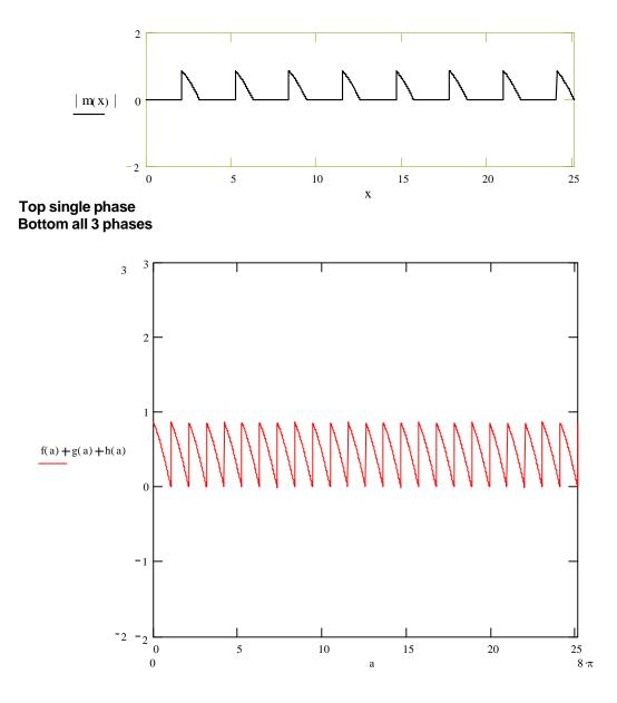
Notice that at 120 degrees, the base of the waveform (the sum of the three rectified phases) is at zero.
